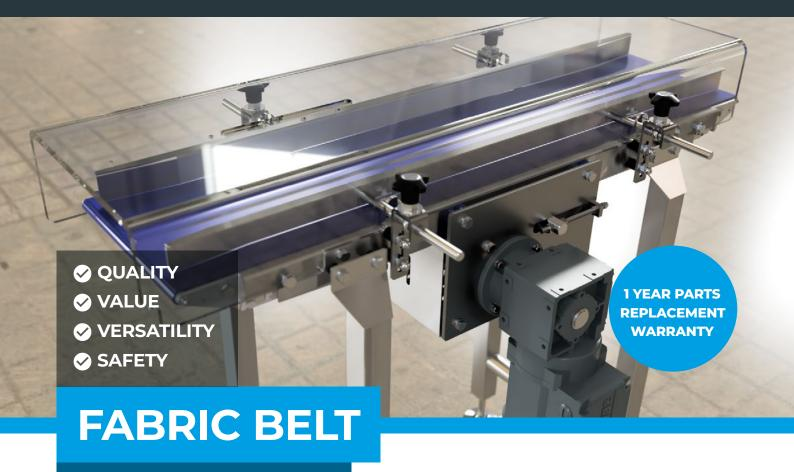
The fabric belt conveyor, with full length adjustable side guides and centre drive to aid small diameter transfer.
